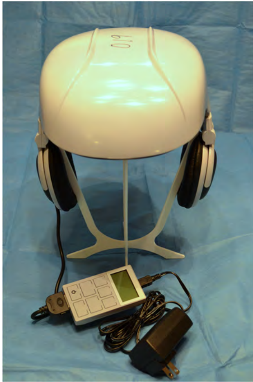
Fig. 1. The TOPHAT655 device unit exterior view. An example of the experimental device is shown with the control unit and power cord attached. Note that there are no identifying markings on the unit with the exception of the device number which is written on the top of the unit.
